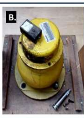
B - Hladinomer Robotron ( ^{60}\text{Co} , ^{137}\text{Cs} )
